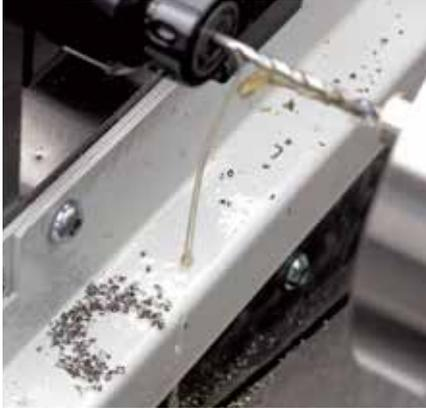
Deep hole drilling with an oil hole drill
