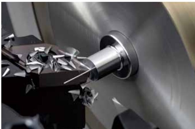
Micromachining leaving 0.2 mm dia. pin
